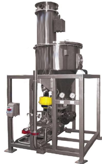
Schenck Process to control the mass ratio of product to gas and correct air flow adjustments with extraordinary precision. The Macturi keeps the system stable even under turbulent conditions.
