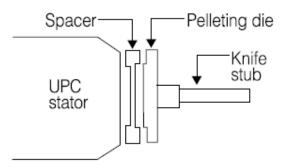
As the pellet leaves the die, a variable-speed rotary cutter controls the pellet length. For example, by increasing the cutter speed, short pellets and crumbles are produced; and by reducing cutter speed, longer pellet lengths are produced. This flexibility eliminates the need for crumbling rolls to produce a crumbled feed.
