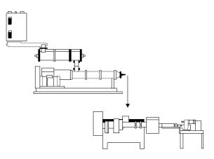
This processing system has the advantage of being able to operate both extruders at their maximum rate potential. When only one extruder is used to produce a very dense pellet, the extruder may have to be operated at lower throughputs to prevent expansion. Adding the second forming extruder (PDU) can allow a feed manufacturer to produce a wide range of feed densities from highly-expanded feeds with one extruder, or very dense feeds with the cooking extruder and PDU.
